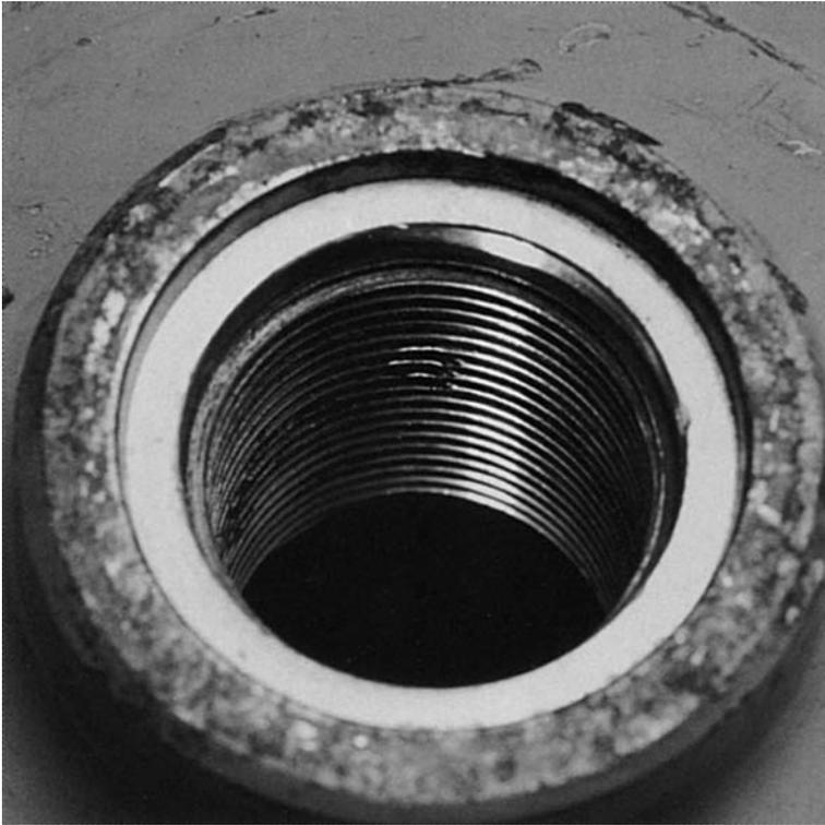
**PHOTO 5.** Damaged threads. This damage is easily seen with the naked eye, but the thread area is dirty and first needs cleaning (see NOTE 9), before proceeding with the visual inspection of the thread area.
